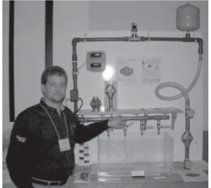
Dye shows the movement of containments through the ground water flow model that was on display at the conference.
