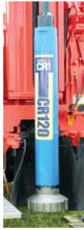
The Cyclops™ bit is mounted on this 12-inch diameter Center Rock CR120 down-the-hole hammer that has a piston that weighs a whopping 304 pounds.
