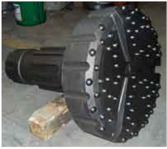
This Center Rock 20-inch Cyclops™ button bit was use to drill the top hole.
